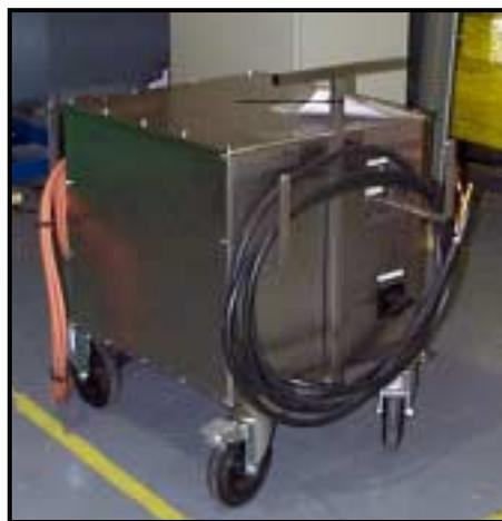
**Figure 7.23 Typical Helicopter Start Facility**
