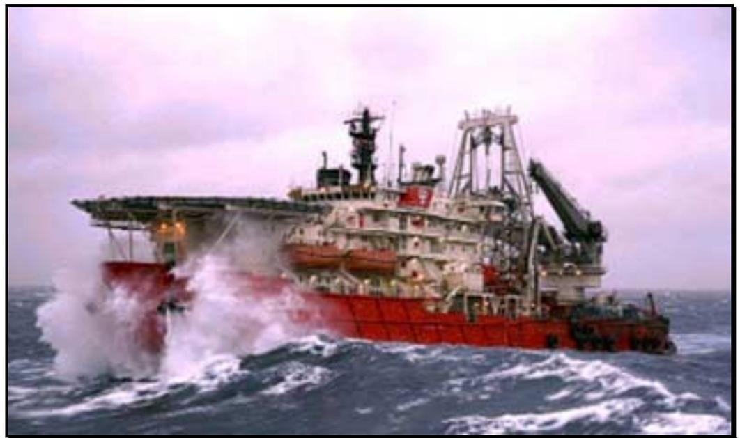
**Figure 8.1 Example of a Helideck Severely Affected by Vessel Motions**
